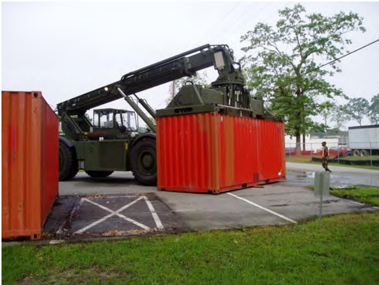
A rough terrain cargo handler (RTCH) maneuvers a container into position for the 719th. 2002.
