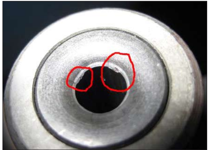
Above: Even slight damage to a barrel’s crown reduces accuracy. The lands in a rifled barrel are about the same height as the thickness of a piece of paper. Stop wrecking your small arms!
