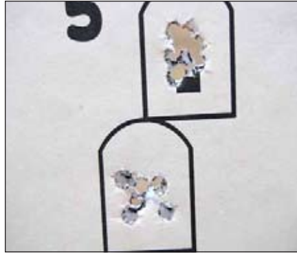
Above: A good gunner can produce a centered, circular cone of fire no larger than four mils. The pasters on 10 meter target are four centimeters wide, which is four mils at that distance.
